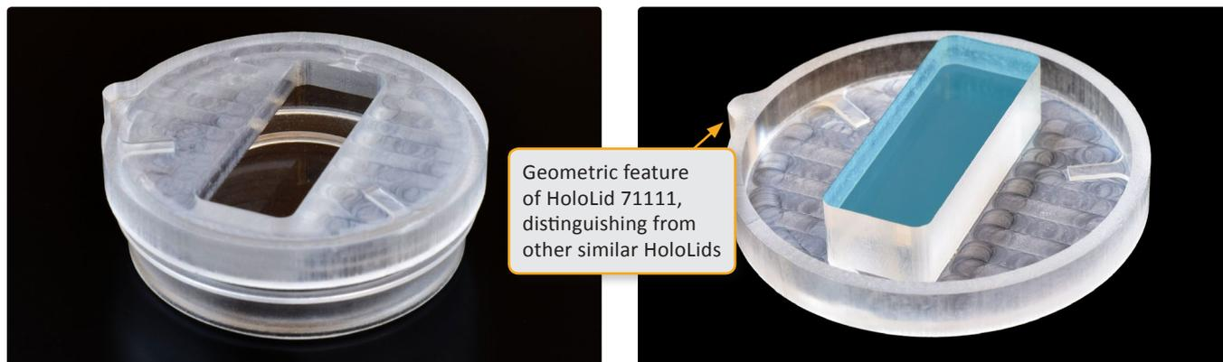
HoloLid placed on a ibidi  $\mu$ -Dish 35 mm, high (left). The area marked blue is the observation window which is immersed into the cell media (right).
